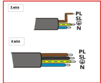
**4-wire switchable with emergency light function in case of a power failure.**
